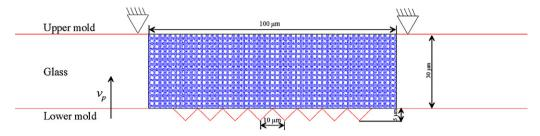
Fig. 2. Two-dimensional simulation model for GMP of microgrooves.
