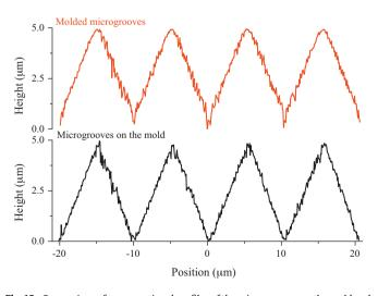
**Fig. 12.** Comparison of cross-sectional profiles of the microgrooves on the mold and those on the molded glass plate.
