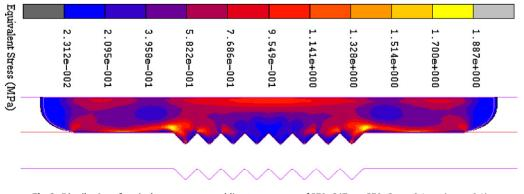
**Fig. 3.** Distribution of equivalent stress at a molding temperature of 570 °C ( $T_{mid}$  = 570 °C,  $v_p$  = 0.1 mm/s,  $\mu_f$  = 0.1).
