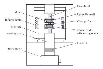
Fig. 7. Schematic diagram of the structure of the ultraprecision glass molding machine.
