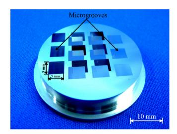
Fig. 8. Photograph of the Ni–P mold with microgrooves.
