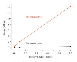
Fig. 5. Change of stress with pressing velocity.
