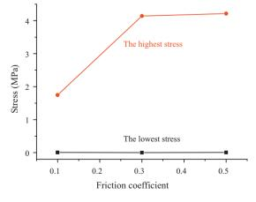
Fig. 6. Change of stress with friction coefficient.
