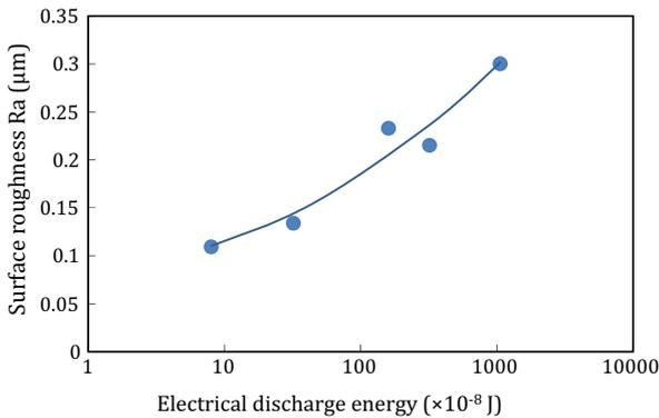
Fig. 7. Change in PCD surface roughness with discharge energy.
