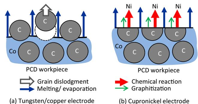
Fig. 1. Surface formation mechanisms of PCD in EDM using (a) conventional electrodes and (b) cupronickel electrodes.
