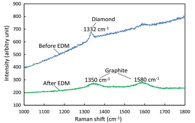
Fig. 9. Raman spectra of PCD before and after EDM.
