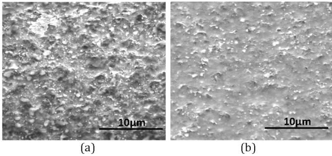
Fig. 6. SEM micrographs of surfaces machined using (a) tungsten block electrodes and (b) cupronickel wheel electrodes.
