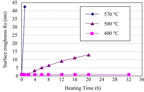
**Figure 4** Influence of mould surface structure on surface roughness change of the mould during heating (see online version for colours)
