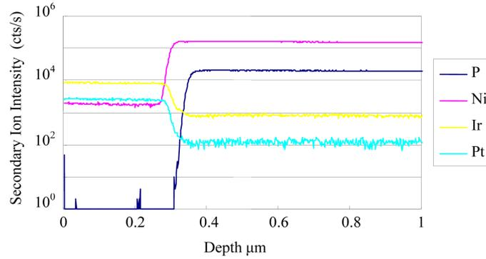
**Figure 7** Cross-sectional photograph and depth profile of the mould composition: (a) schematic diagram before heating; (b) TEM image and (c) depth profile after heating at 570°C for 1 h (see online version for colours)
