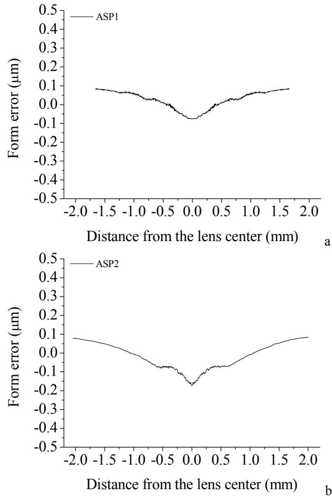
Figure 5. Form error profiles of a molded lens: (a) upper surface ASP1, (b) lower surface ASP2.
