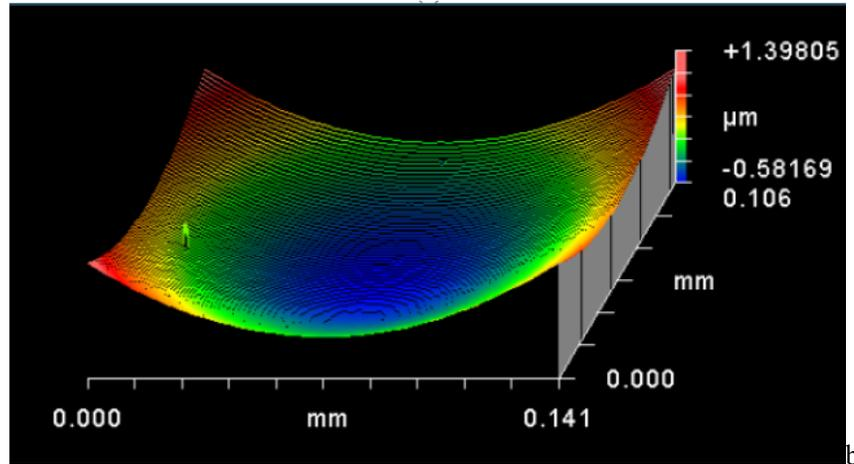
Figure 10. Three-dimensional measurement results of the molding dies after 100 GMP shots: (a) upper die, (b) lower die.
