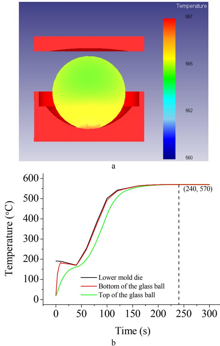
Figure 11. FEM simulation results of temperature distribution and temperature changes in the glass ball and the molding dies during heating: (a) temperature distribution, (b) temperature changes with time.
