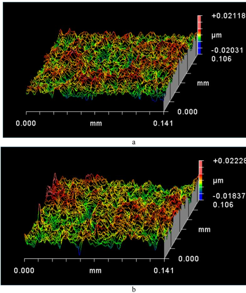
Figure 7. Microscopic topographies of the molded aspherical lens after removing the aspherical curvature: (a) upper surface ASP1, (b) lower surface ASP2.
