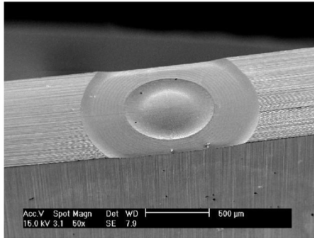
**Figure 14** Optical microscope image of a shaped convex spherical surface on tungsten carbide
