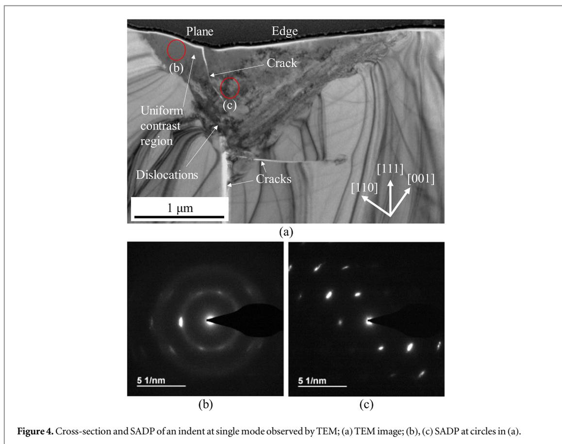
**Figure 4.** Cross-section and SADP of an indent at single mode observed by TEM; (a) TEM image; (b), (c) SADP at circles in (a).
