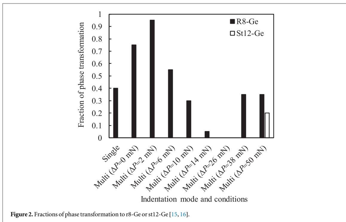
Figure 2. Fractions of phase transformation to r8-Ge or st12-Ge [15, 16].
