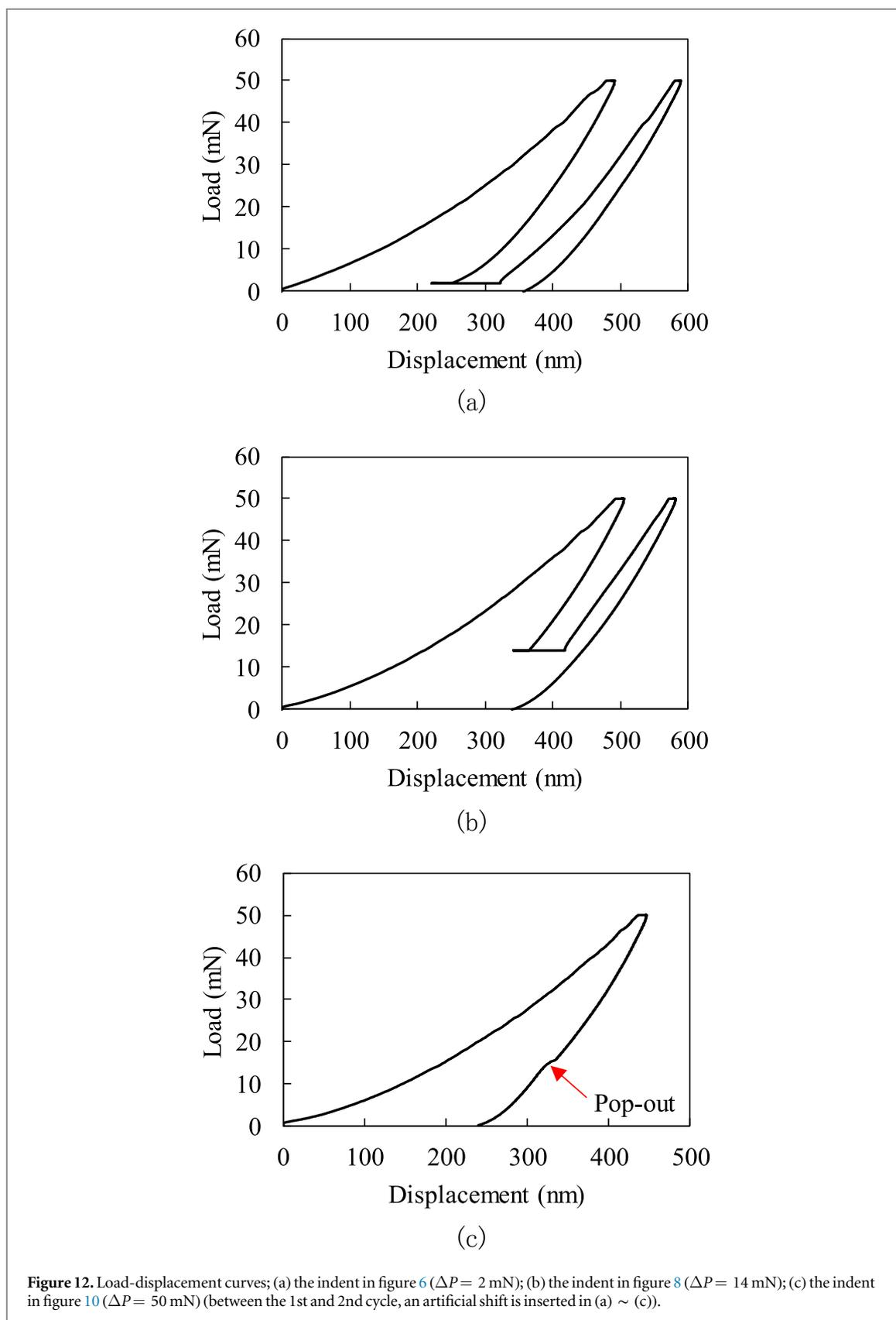
**Figure 12.** Load-displacement curves; (a) the indent in figure 6 ( $\Delta P = 2$  mN); (b) the indent in figure 8 ( $\Delta P = 14$  mN); (c) the indent in figure 10 ( $\Delta P = 50$  mN) (between the 1st and 2nd cycle, an artificial shift is inserted in (a) ~ (c)).
