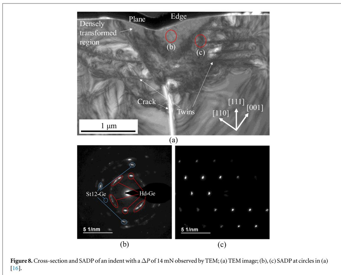
**Figure 8.** Cross-section and SADP of an indent with a  $\Delta P$  of 14 mN observed by TEM; (a) TEM image; (b), (c) SADP at circles in (a) [16].
