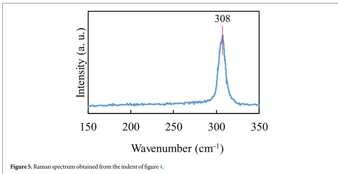
**Figure 5.** Raman spectrum obtained from the indent of figure 4.
