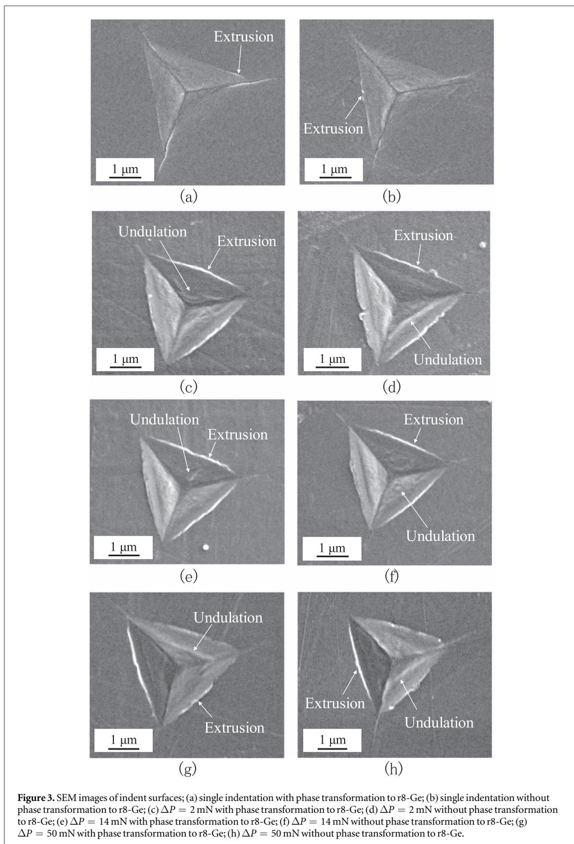
and the amount of each phase is not enough to appear on Raman spectra. Therefore, the plastic flow is not an indication of end phases on Raman spectra. To reveal the different phase transformation mechanism depending on indentation conditions, behaviors beneath the surface should be investigated.
