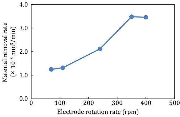
Fig. 5. Change in material removal rate with electrode rotation rate.
