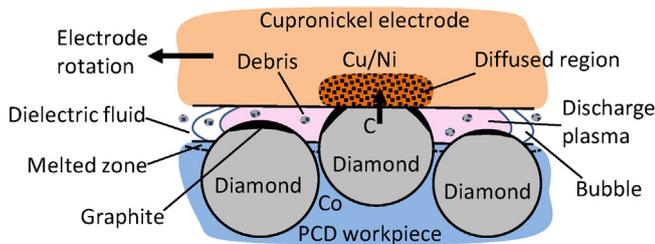
Fig. 11. Schematic model of interfacial phenomena between PCD workpiece and cupronickel electrode in EDM.
