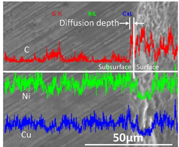
Fig. 10. EDX analysis result of a cupronickel electrode, showing diffusion of the C element from PCD to cupronickel.
