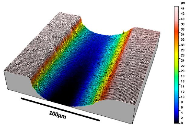
Fig. 8. Three-dimensional topography of a microgroove on PCD machined using a cupronickel wheel electrode.
