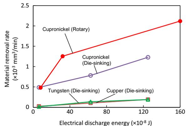
Fig. 4. Material removal rates for different types of electrodes.
