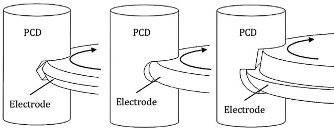
Fig. 2. Schematic of EDM using rotary cupronickel electrodes having various cross-sectional shapes.
