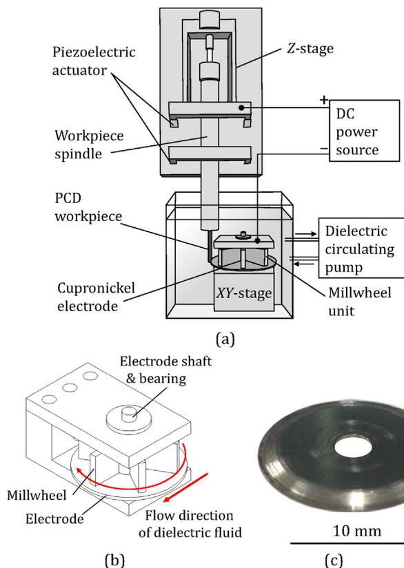
Fig. 3. The developed prototype  $\mu$ -EDM setup: (a) system diagram, (b) rotary electrode unit, and (c) cupronickel electrode.
