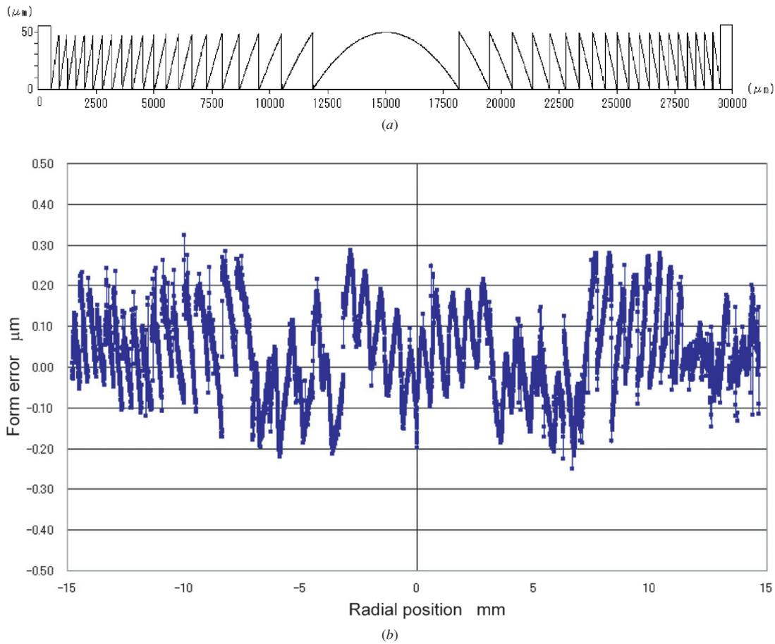
**Figure 8.** Two-dimensional measurement results of the lens geometry: (a) cross-sectional profile, (b) form error distribution.
