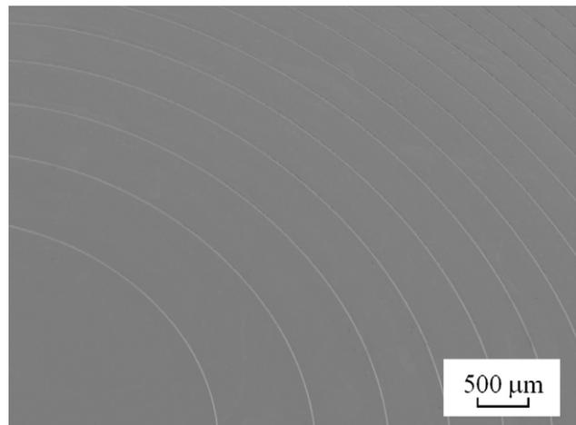
**Figure 6.** Scanning electron micrograph of the fabricated Fresnel lens.
