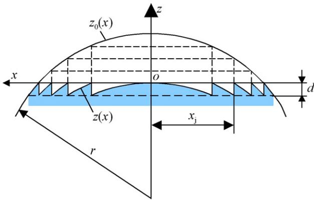
**Figure 1.** Schematic of the geometry of a Fresnel lens.
