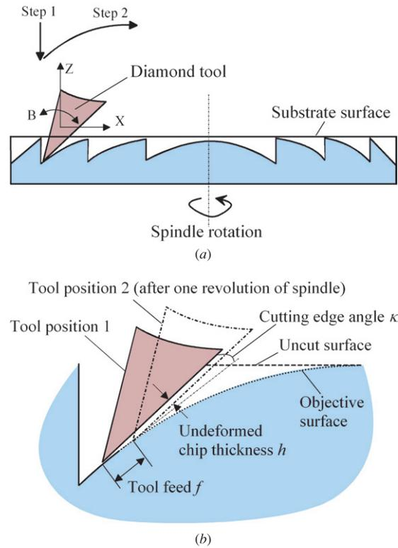
**Figure 2.** Machining models for the Fresnel structures: (a) process steps, (b) ductile machining model of a single microgroove.
