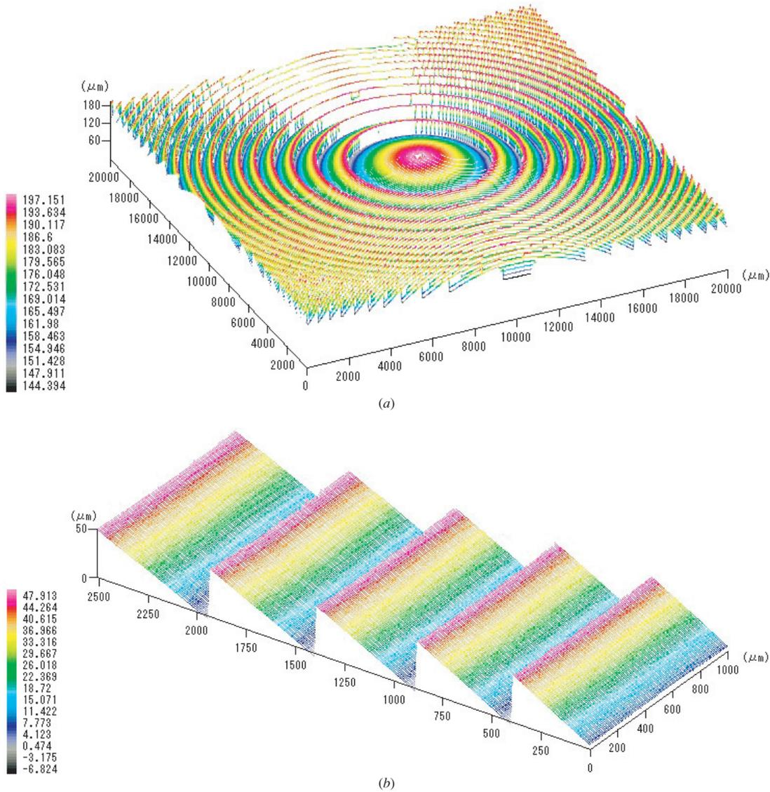
Figure 7. Three-dimensional topographies of the lens: (a) central region, (b) outer region.
