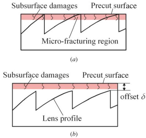
**Figure 3.** The depth-offsetting method to avoid the influences of precut-induced damaged layer.
