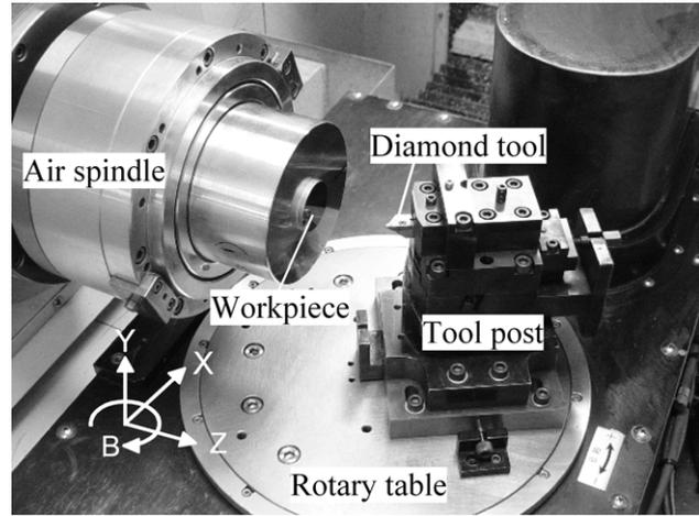
**Figure 4.** Photograph of the main section of the ultraprecision lathe.
