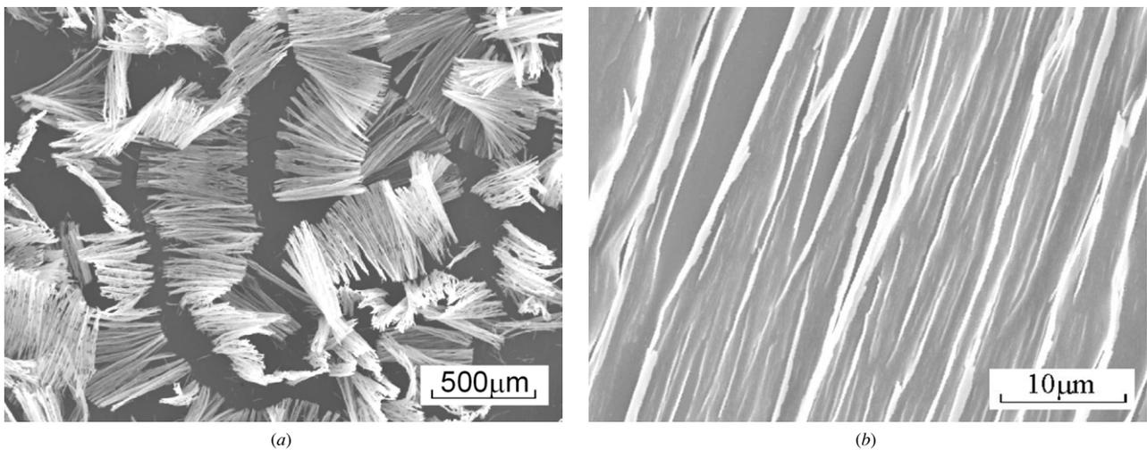
**Figure 9.** Scanning electron micrographs of the cutting chips: (a) general view, (b) detailed view.
