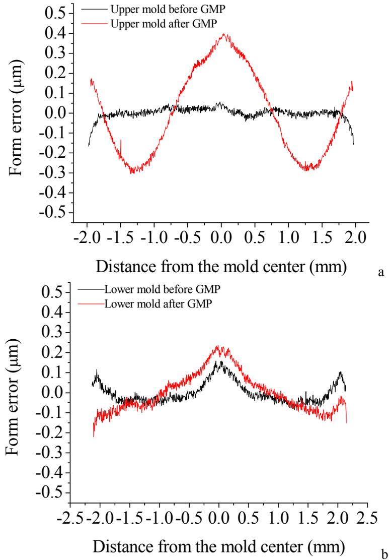
Figure 8. Changes in form error profile of the molding dies after 100 GMP shots: (a) upper die, (b) lower die.
