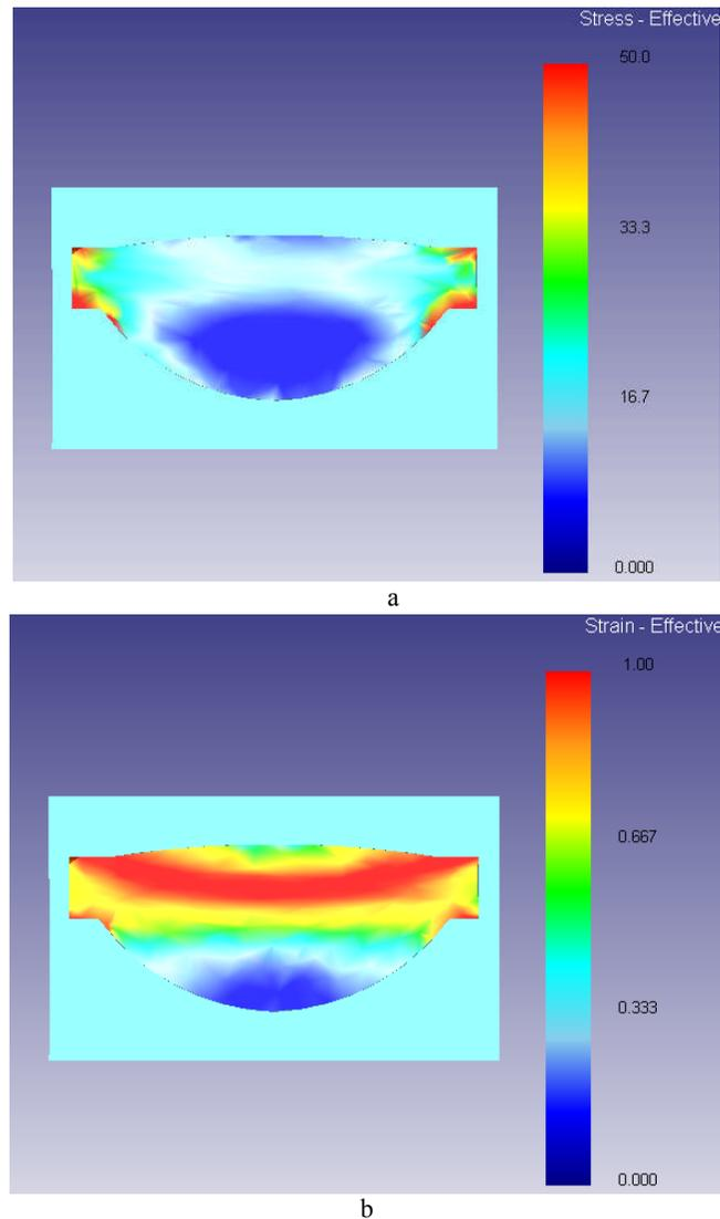
Figure 12. Distributions of (a) stress and (b) strain in the molded glass lens at a molding temperature of 570°C.
