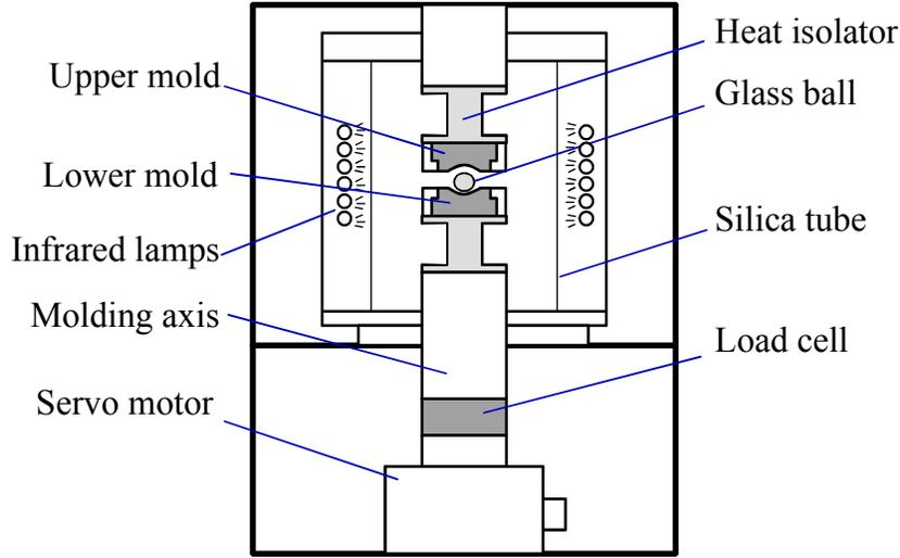
Figure 1. Schematic of the configuration of the ultraprecision glass molding machine.
