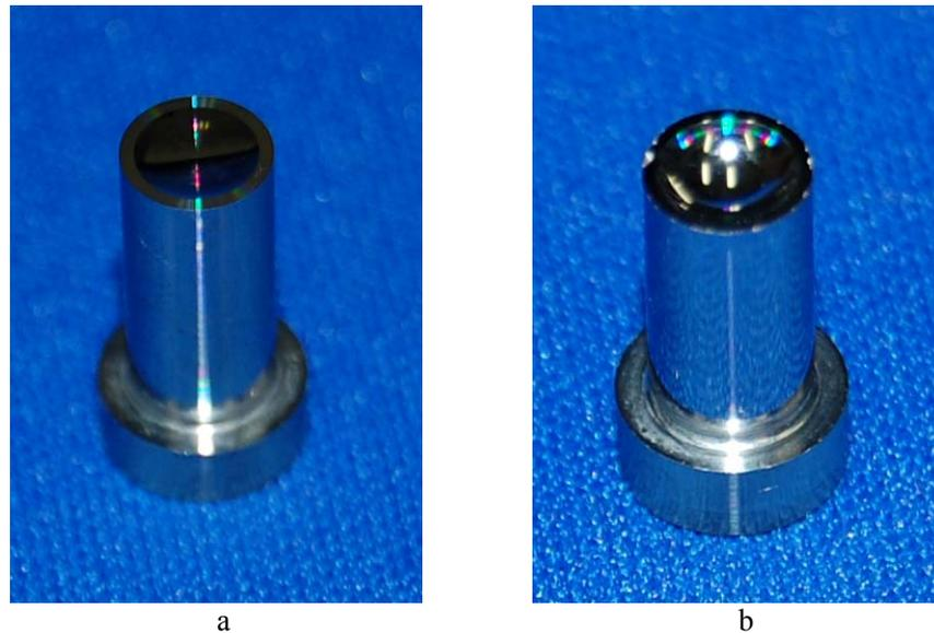
Figure 3. Photographs of the molding dies for GMP tests: (a) upper die, (b) lower die.
