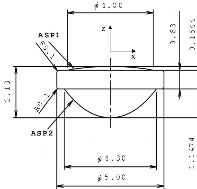
Figure 2. Shape of the objective biconvex aspherical glass lens.
