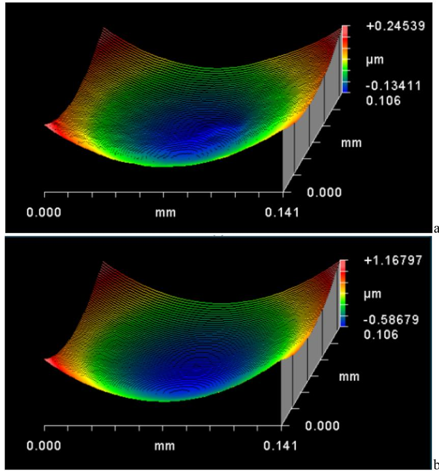
Figure 9. Three-dimensional measurement results of the molding dies before GMP experiments: (a) upper die, (b) lower die.
