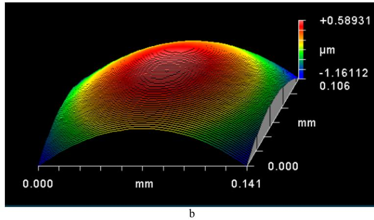
Figure 6. Three-dimensional measurement results of the center region of a molded lens: (a) upper surface ASP1, (b) lower surface ASP2.
